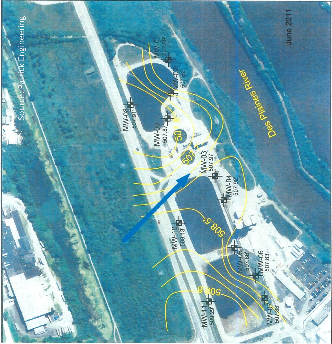
Figure 3 June 2011 Second Quarter Ground-water Contours Showing Mounding Beneath the Joliet Ash Ponds (PCB 2013-015)
